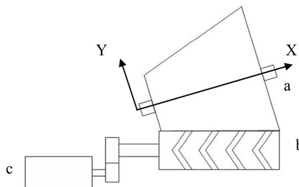
Fig. 1 — Random cone system [(a) conical package, (b) grooved drum and (c) motor]
