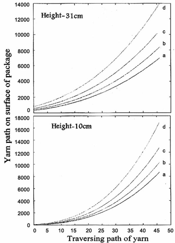
Fig. 4 — Yarn curvature for different heights of concentration point and various start angles of winding [(a) 60°, (b) 65°, (c) 70° and (d) 75°]
