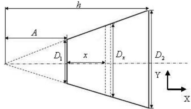
Fig. 2 — Cone dimensions [ $D_1$ — nose diameter,  $D_2$ — base diameter,  $D_x$ — diameter in  $x$  point,  $h$ — height of cone, and  $A$ — distance between concentration point and nose]
