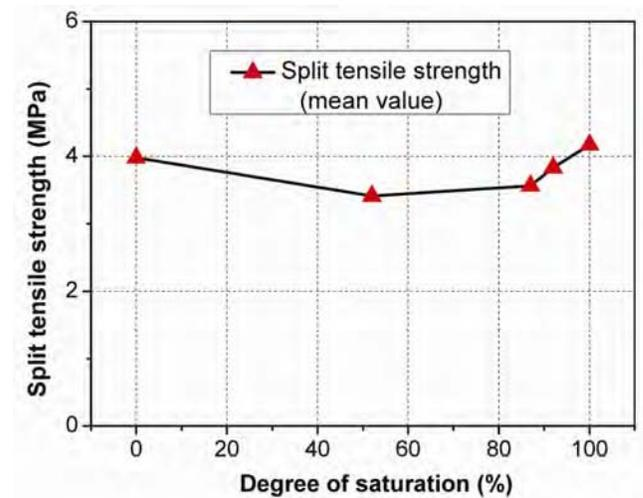
Fig. 8—Effect of degree of saturation on split tensile strength (mean values)
