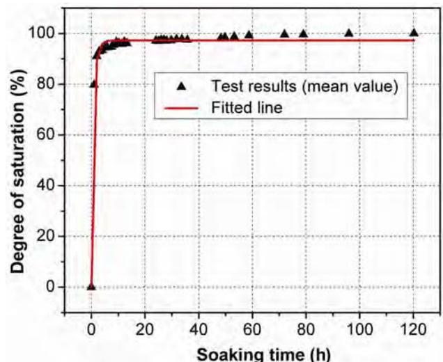
Fig. 6—Variation of degree of saturation ratio during soaking process
