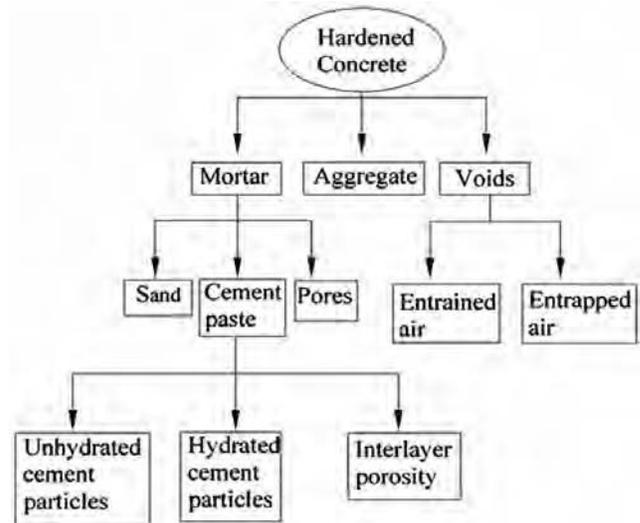
Fig. 1—Typical phases of hardened concrete
