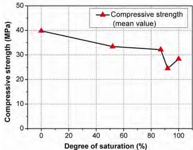
Fig. 7—Effect of degree of saturation on compressive strength (mean values)
