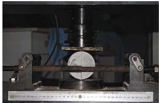
Fig. 4—Split tensile testing system layout
