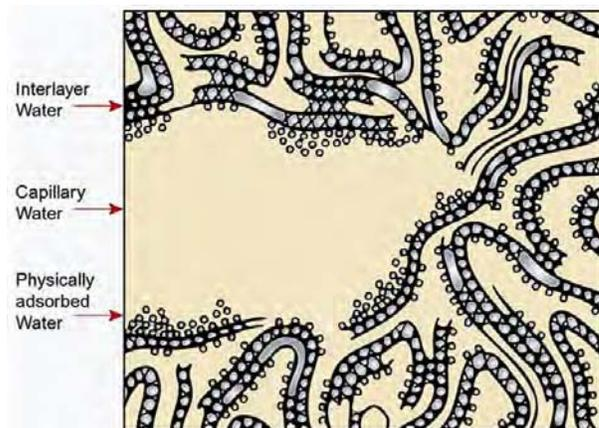
Fig. 2—Diagrammatic model of the water type in concrete (adapted from Metha and Monteiro<sup>22</sup>)
