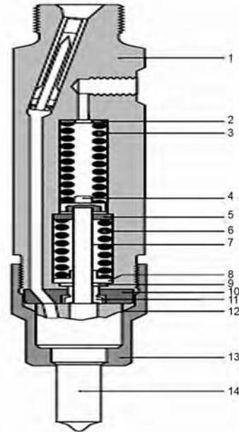
Fig. 1—Two-springs injector [1 – nozzle-holder body, 2 – shim, 3 – spring, 4 – pressure pin, 5 – guide element, 6 – spring 2, 7 – pressure pin, 8 – spring seat, 9 – shim, 10 – intermediate element, 11 – stop sleeve, 12 – nozzle needle, 13 – nozzle-retaining nut, 14 – nozzle body]
