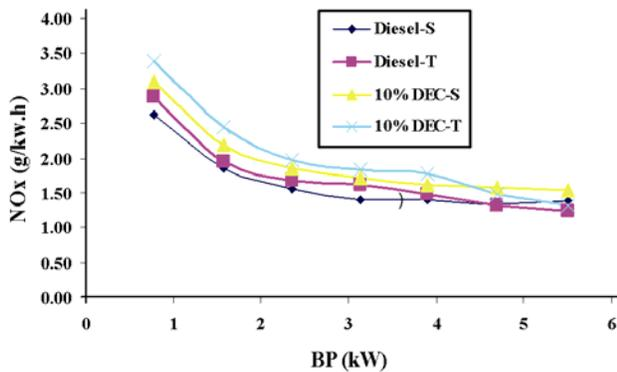
Fig. 6—Comparison of oxide of nitrogen (NOx) of 10%DEC oxygenated diesel blend between standard single-spring injection and two-springs split injection
