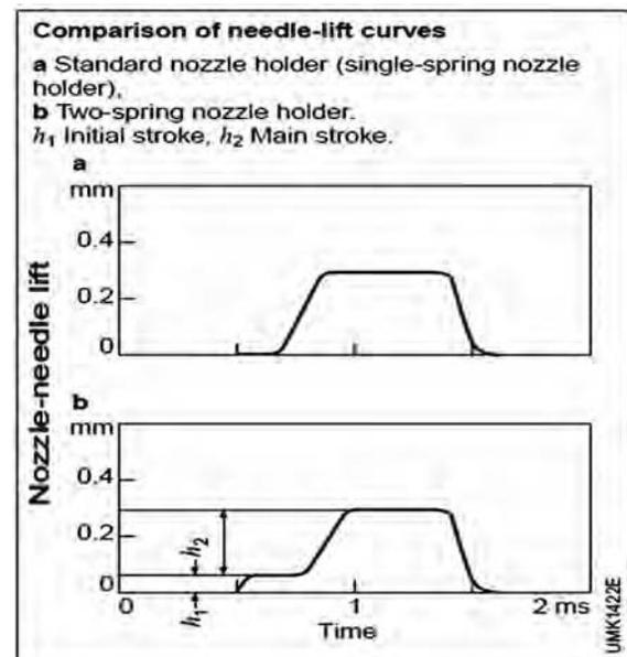
Fig. 2—Comparison of needle lift
