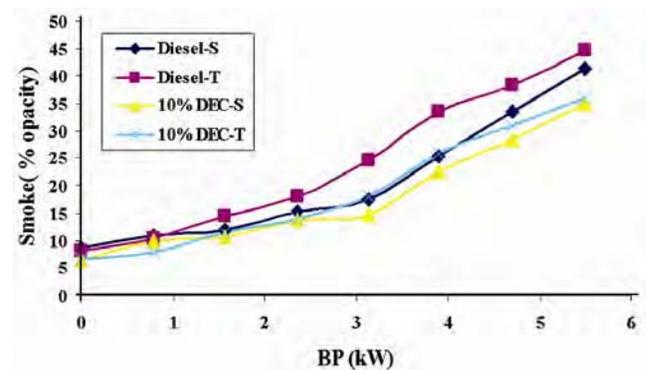
Fig. 8—Comparison of smoke opacity of 10%DEC oxygenated diesel blend between standard single-spring injection and two-springs split injection
