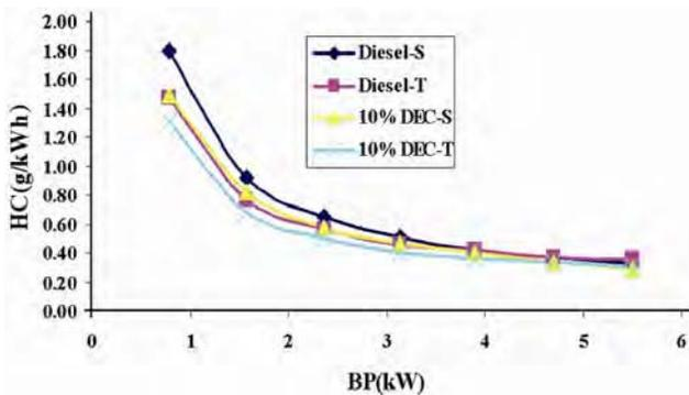
Fig. 5—Comparison of hydrocarbon (HC) of 10%DEC oxygenated diesel blend between standard single-spring injection and two-springs split injection
