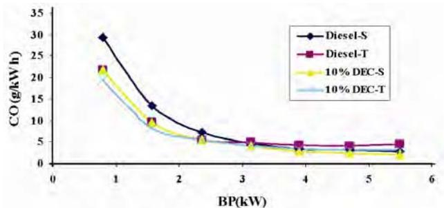
Fig. 4—Comparison of carbon monoxide (CO) of 10%DEC oxygenated diesel blend between standard single-spring injection and two-springs split injection
