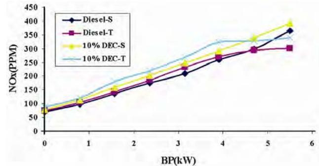
Fig. 7—Comparison of oxide of nitrogen (NOx) (ppm) of 10%DEC oxygenated diesel blend between standard single-spring injection and two-springs split injection
