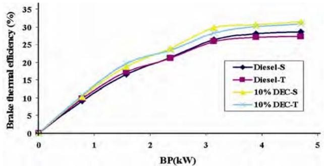
Fig. 3—Comparison-of brake thermal efficiency of 10%DEC oxygenated diesel blend between standard single-spring injection and two-springs split injection
