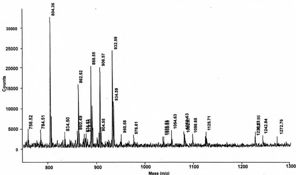
Fig. 1—Mass spectrometric spectrum of peptides obtained following PVDF membrane purification of tryptic peptides extracted after *in-gel* enzymic (trypsin) digestion. [All the signals with masses indicated correspond to tryptic peptides (only the mass region of  $m/z$  750 to 1300 is shown)]
