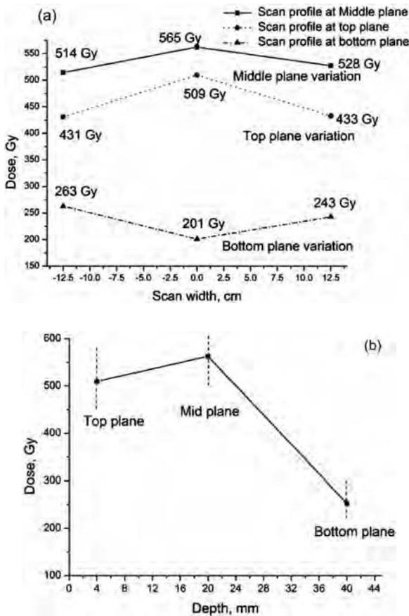
Fig. 3 — (a) Scan profiles in all the planes of the product box (depth 40 mm), (b) depth dose profile for one sided irradiation in semolina medium
