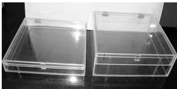
Fig. 1 — Dummy product boxes made of Perspex with depth 40 mm and 90 mm for 10 MeV e-beam food irradiation dosimetry experiments
