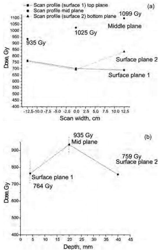
Fig. 4 — (a) Scan profiles in all the planes of the product box (depth 40 mm) and (b) depth dose profile for both sided irradiation in semolina medium
