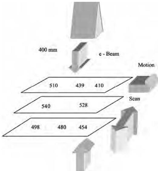
Fig. 2 — Schematic diagram of both sided irradiation geometry of 10 MeV e-beam and distribution of absorbed dose inside the product box containing food sample of bulk density 0.58 g/cc
