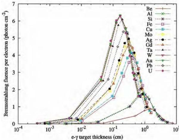
Fig. 1 — Variation in integrated bremsstrahlung fluence as a function of e- $\gamma$  target thickness for 15 MeV electron incidents on different materials
