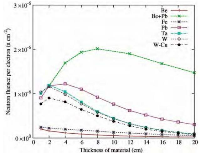
Fig. 2 — Variation in integrated neutron fluence as a function of  $\gamma$ -n target thickness for different materials
