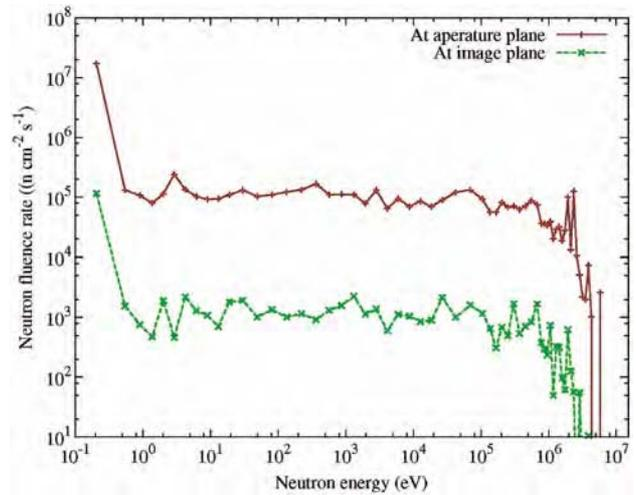
Fig. 6 — Neutron energy spectrum calculated at aperture and image plane for the optimized design of 15 MeV accelerator based neutron radiography facility
