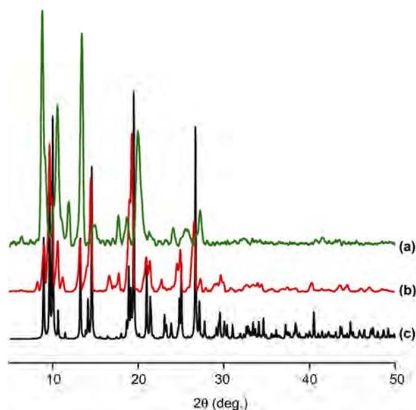
Fig. 6—The PXRD patterns of compound (**1**). [(a) simulated; (b) as-synthesized; (c) heated at 433 K].
