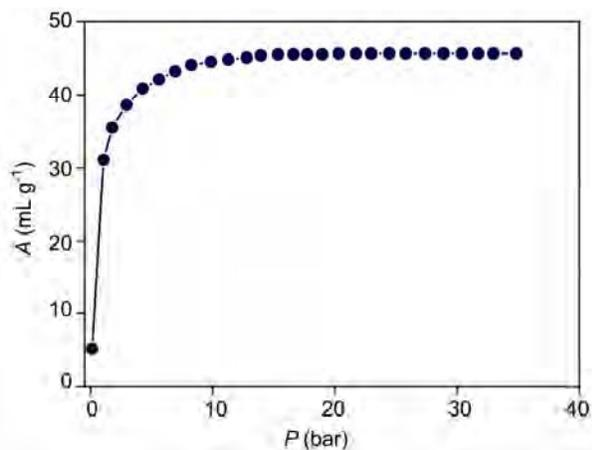
Fig. 8—CO<sub>2</sub> adsorption profile at 298 K up to 40 bar pressure.
