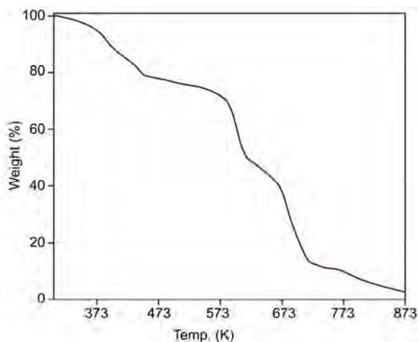
Fig. 5—TGA curve for compound (**1**) under N<sub>2</sub> atmosphere in the temperature range of 30–600 °C.
