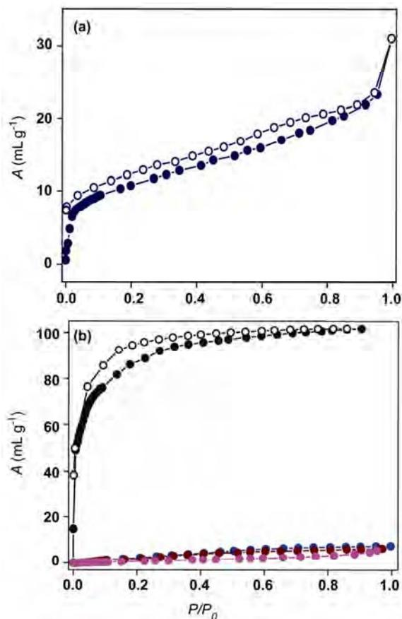
Fig. 7—(a) N<sub>2</sub> adsorption isotherm of (**1'**) at 77 K, and (b) CO<sub>2</sub> (black), N<sub>2</sub> (blue), H<sub>2</sub> (pink) and Ar (wine) gas adsorption isotherms at 195 K. [Adsorption: filled circles; Desorption: open circles].
