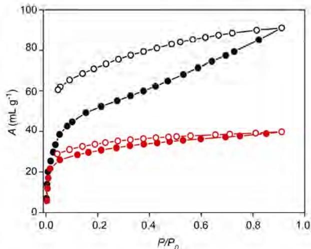
Fig. 9—Benzene (red) and acetonitrile (black) solvent vapour adsorption profiles of (**1'**) at 298 K. [Adsorption: filled circles, Desorption: open circles].
