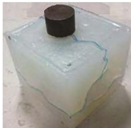
Fig. 5—Silicone rubber mold of a cylinder head (Blue lines indicate the path for cutting the silicone rubber mold)
