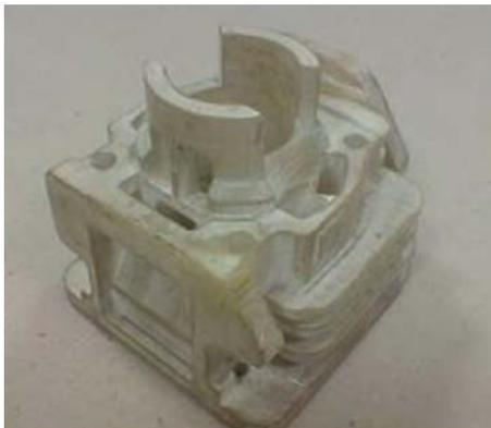
Fig. 4—Cylinder head fabricated by RP machine
