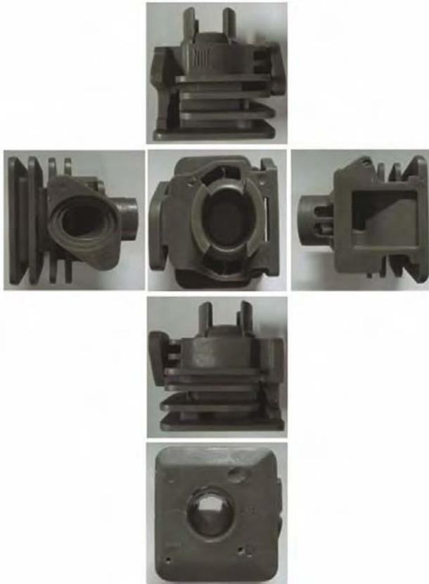
Fig. 9—Wax patterns made from silicone rubber mold
