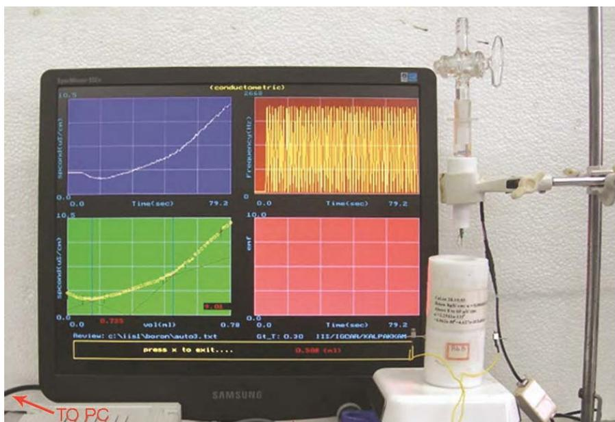
Fig. 1—Photograph of a laboratory made conductometric titration facility used for assay of boron at ppm and sub-ppm levels
