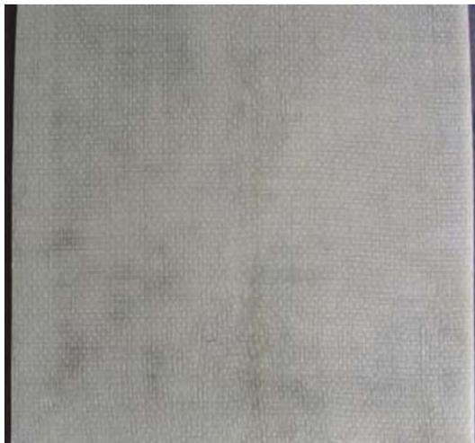
Fig. 2—The fabricated GFRP plate
