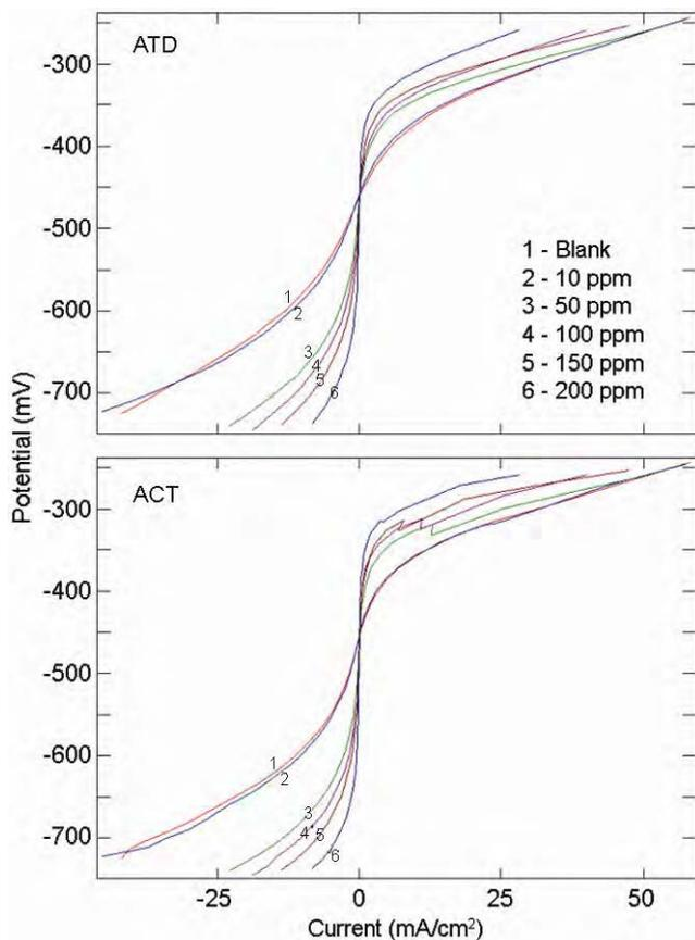
Fig.3—LPR plots for MS in 0.5M HCl in presence of different concentrations of ATD & ACT at 300K
