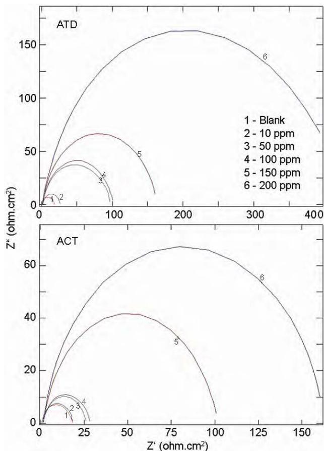
Fig. 4—Nyquist plots of MS in 0.5M HCl in presence of different concentrations of ATD & ACT at 300K
