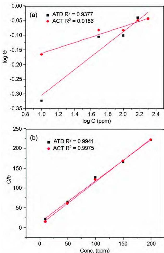
Fig.6—Temkin isotherm (a) and Langmuir isotherm (b) of ATD and ACT on surface of mild steel in 0.5M HCl at 300 K
