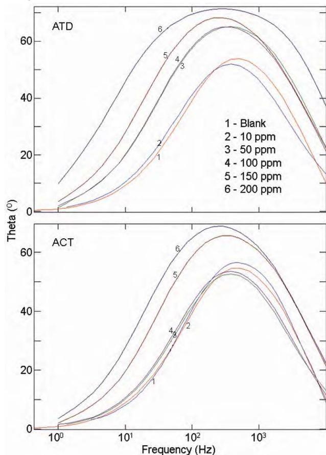
Fig.5—Bode plots of MS in 0.5M HCl in presence of different concentrations of ATD & ACT at 300K
