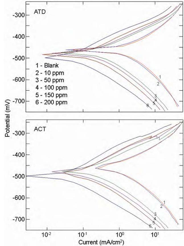
Fig. 2—Polarization curve of MS in 0.5 M HCl in presence of different concentrations of ATD & ACT at 300K
