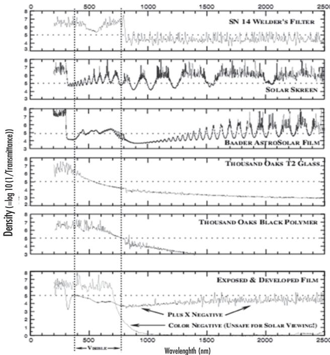
Fig. 1. Spectral Response Curve of filters
