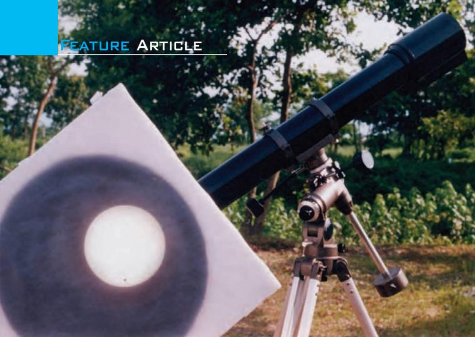
Fig 5. Eyepiece projection. Back projection of ToV 2004 inside a sealed projection funnel. (Picture: Debasis Sarkar)
