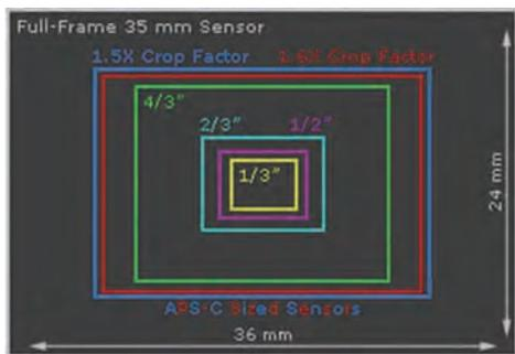
Fig. 4. Different CCD/CMOS panel dimensions
