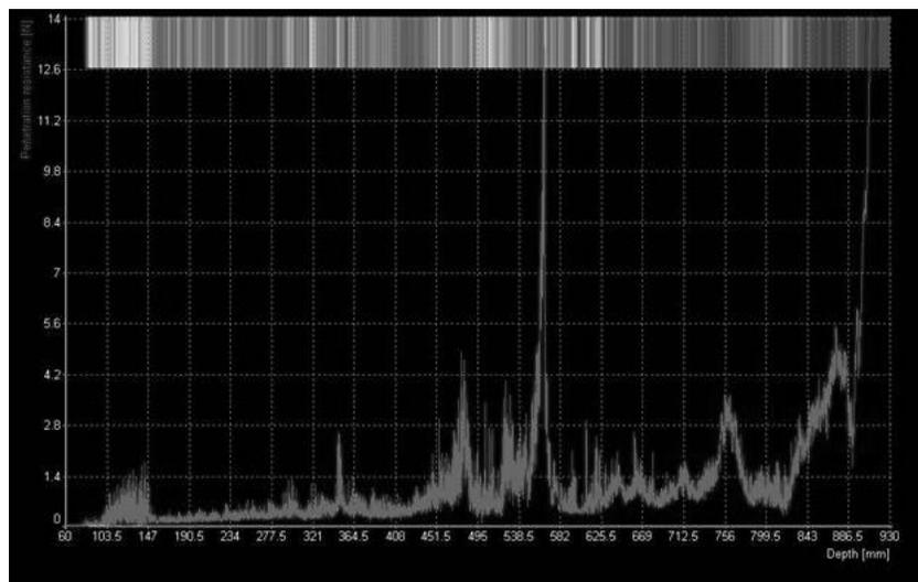
Fig. 3—Force-resistance plot of natural snowpack measured by SMP
