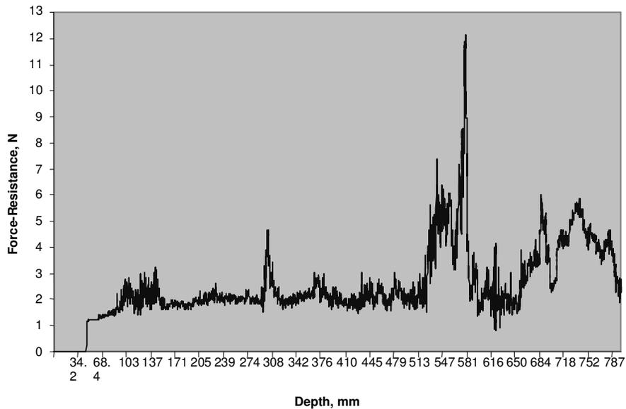
Fig. 2—Force-resistance plot of natural snowpack measured by CSIO developed MPP
