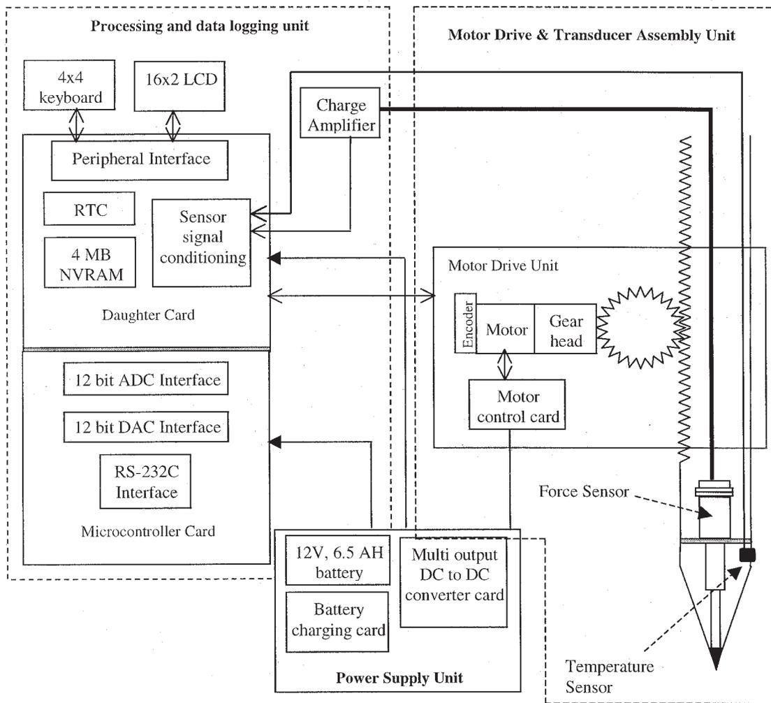
Fig. 1—Block diagram of Multi Parameter Probe (MPP)
