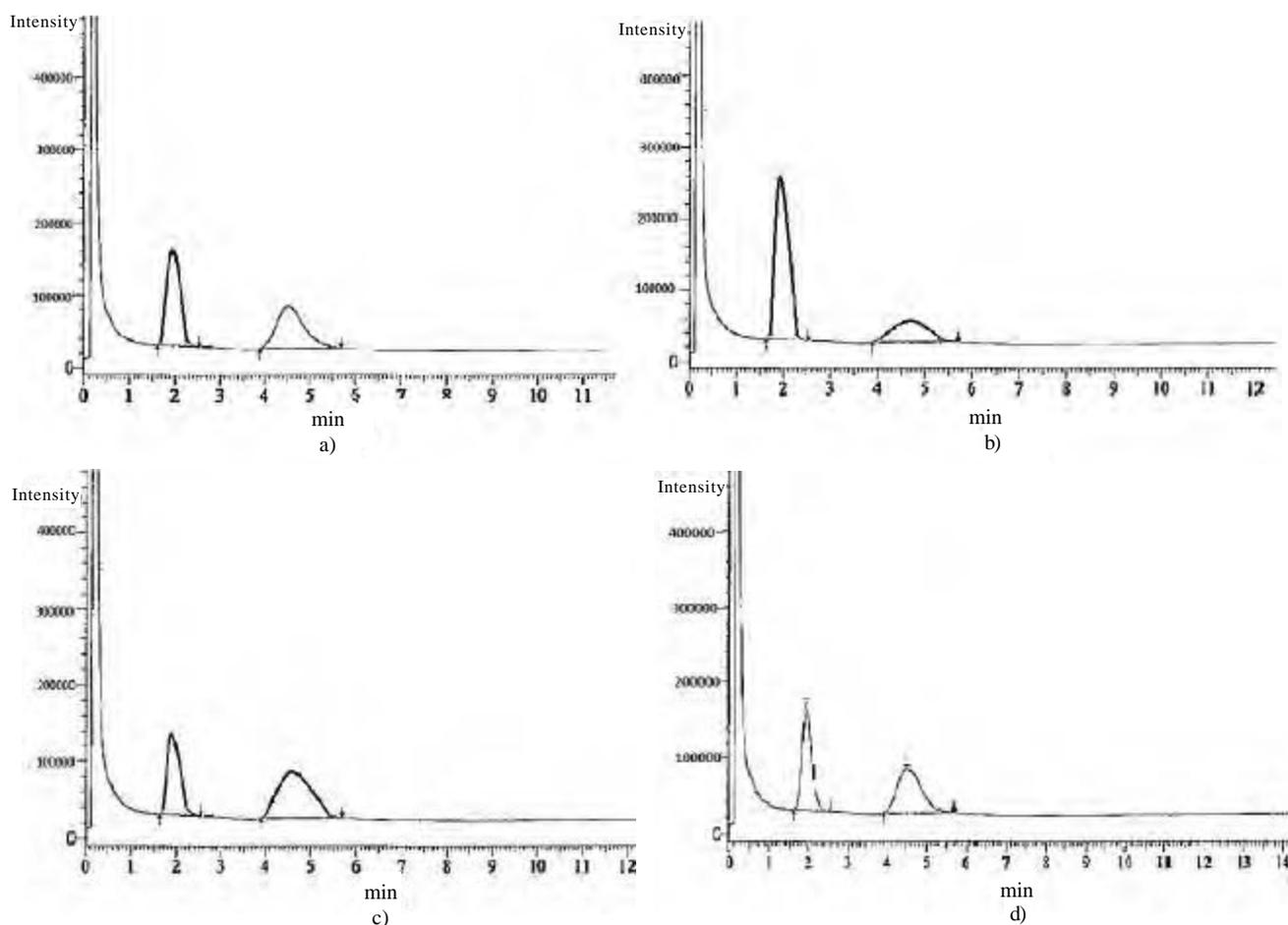
Fig. 3—Analysis of biogas composition by gas chromatography for: a) Sample A; b) Sample B; c) Sample C; and d) sample D
