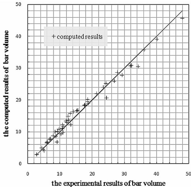
Fig. 7—Comparison of the computed result with the experimental result for the bar ( $10^{-2} \text{ m}^3/\text{m}$ )
