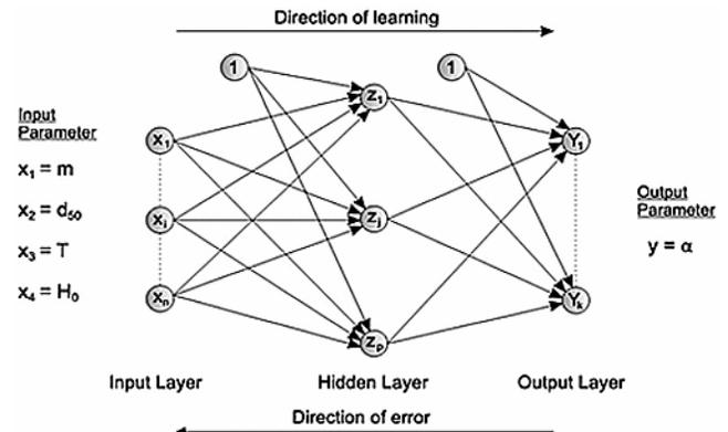
Fig. 3—The architecture of back-propagation network model
