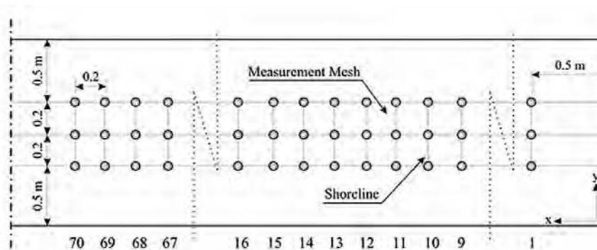
Fig 5—Measurement mesh in the wave flume<sup>9, 10, 41</sup>
