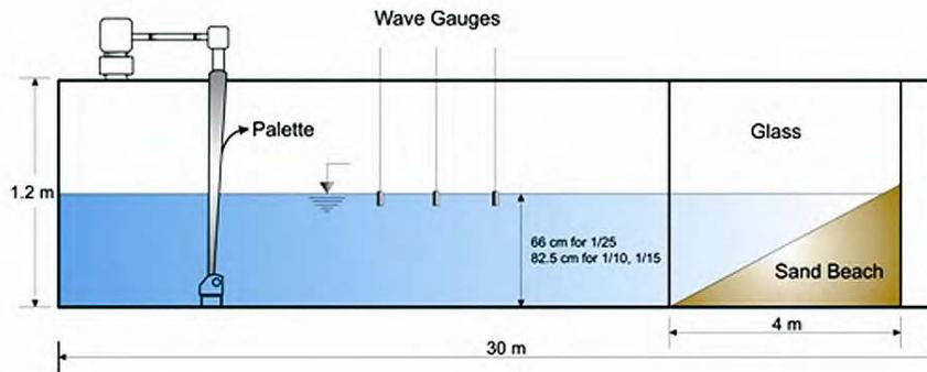
Fig 4—The regular wave flume<sup>9, 10, 41</sup>
