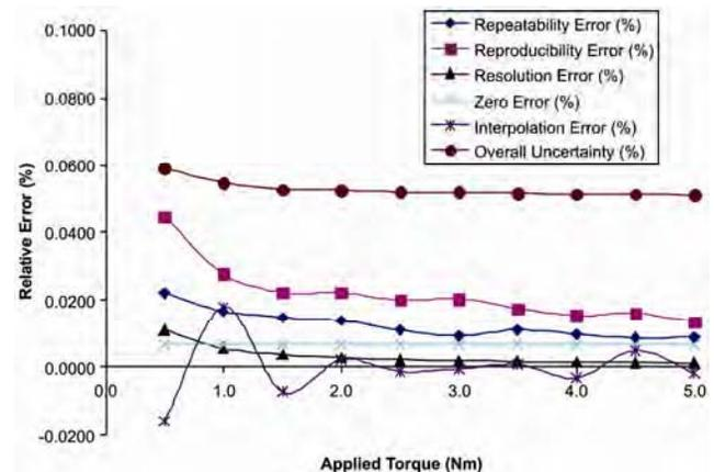
Fig. 4 — Metrological characterization of torque transducer
