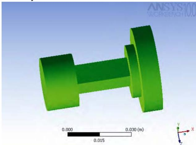
Fig. 1 — Dimensional model of torque sensor
