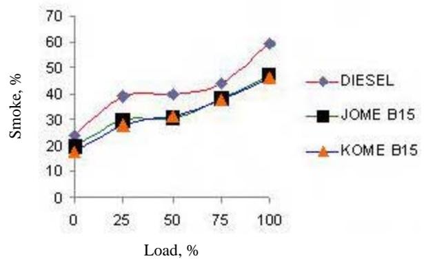
Fig. 6—Smoke for diesel and biodiesel blends
