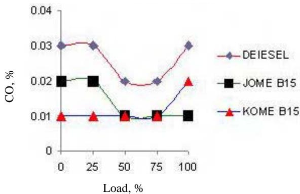
Fig. 5—Carbon monoxide (CO) for diesel and biodiesel blends
