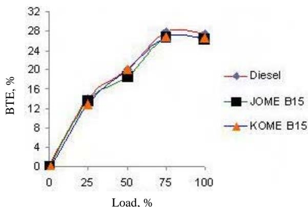
Fig. 1—Brake thermal efficiency for diesel and biodiesel blends
