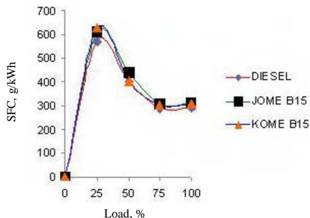
Fig. 2—Brake specific fuel consumption for diesel and biodiesel blends
