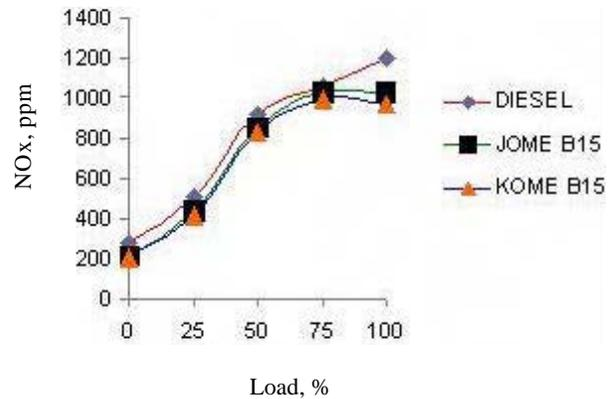
Fig. 4—Oxides of nitrogen (NOx) for diesel and biodiesel blends
