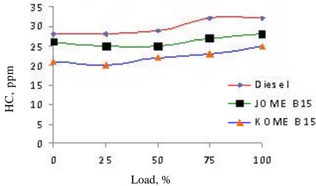
Fig. 3—Hydrocarbon for diesel and biodiesel blends
