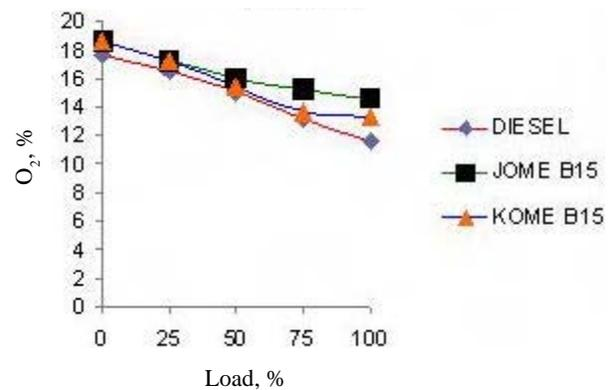
Fig. 7—Oxygen in exhaust for diesel and biodiesel blends
