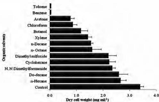
Fig. 1—Dry cell weight of *P. aeruginosa* MTCC 7926 cultured in 100 mL of the nutrient liquid medium (pH 9) and 30 mL of organic solvent at 40°C for 72 h.
