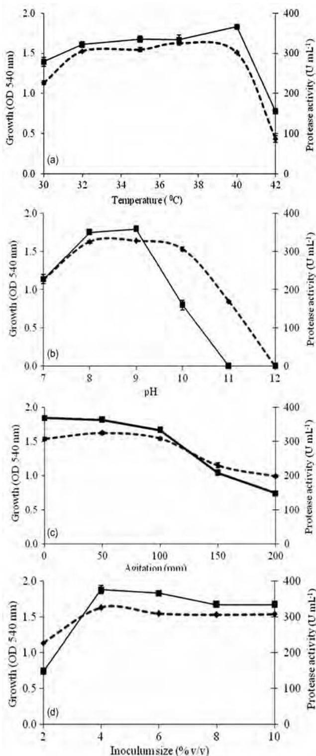
Fig. 3—Effect of physical parameters on the growth and alkaline protease production by *P. aeruginosa*. (a) temperature; (b) pH; (c) agitation; & (d) inoculum.
