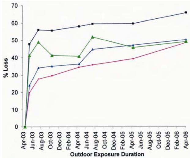
Fig.6—Effect of outdoor exposure on breaking strength (BS) & work of rupture (WOR) of control nylon & polyester webbings [-▲- BS nylon, -▲- WOR nylon, -■- BS polyester and -■- WOR polyester]
