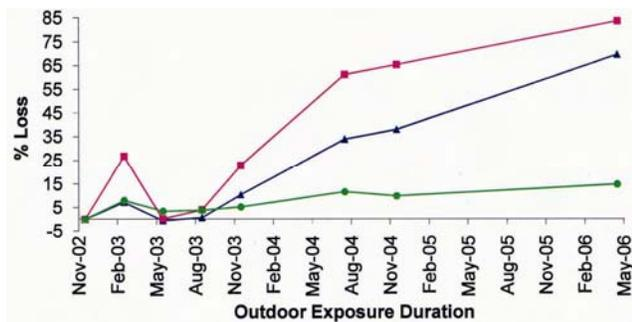
Fig.1—Effect of outdoor exposure on breaking strength, extension-at-break and work of rupture of PU coated nylon fabric (BS specimens) [-▲- Breaking strength, -■- Work of rupture and -●- Extension-at-break]
