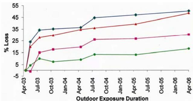
Fig.3—Effect of outdoor exposure on breaking strength of nylon and polyester webbings [-♦- Nylon control, -■- Nylon UVR finished, -▲- Polyester control, -●- Polyester UVR finished]
