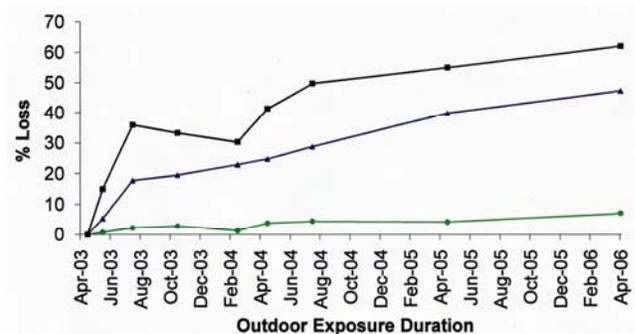
Fig.2—Effect of outdoor exposure on seam shear strength (BS), extension-at-break and work of rupture of PU coated nylon fabric (SSS specimens) [-▲- Breaking strength, -■- Work of rupture and -●- Extension at break]
