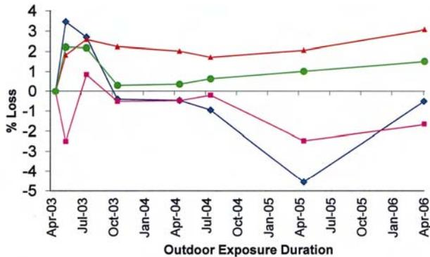
Fig.4—Effect of outdoor exposure on extension-at-break of nylon and polyester webbings [-♦-Nylon control, -■- Nylon UVR finished, -▲- Polyester control and -●- Polyester UVR finished]
