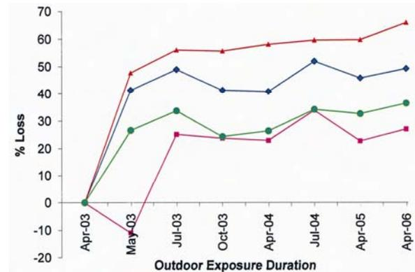
Fig.5—Effect of outdoor exposure on work of rupture of nylon and polyester webbings [-♦- Nylon control, -■- Nylon UVR finished, -▲- Polyester control and -●- Polyester UVR finished]
