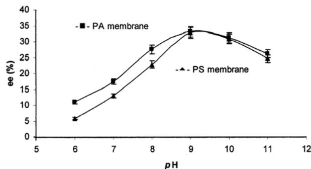
Fig. 2—Change in %ee of *d*-tryptophan with the pH of the feed solution; [BSA] = 0.07% (w/v), and racemic tryptophan =  $3 \times 10^{-3}$  % (w/v).
