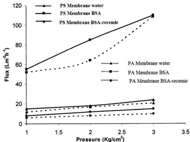
Fig. 5—Permeate flux of membranes for different feeds after 30 min
