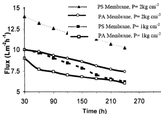
Fig. 6—Permeate flux of membranes with time at pressures 1 and 2 kg/cm<sup>2</sup>
