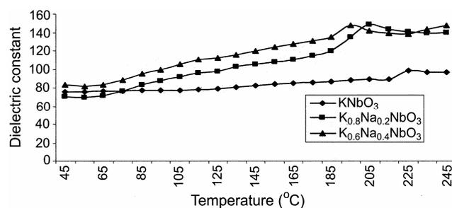
Fig. 2 — Variation of dielectric constant with temperature for  $K_{1-x}Na_xNbO_3$  at 1 MHz
