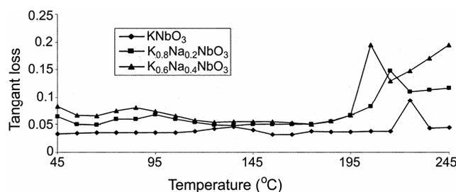
Fig. 4 — Variation of tangent loss with temperature for  $K_{1-x}Na_xNbO_3$  system at 1 MHz
