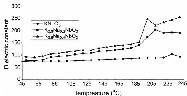
Fig. 3 — Variation of dielectric constant with temperature for  $K_{1-x}Na_xNbO_3$  system at 100 kHz
