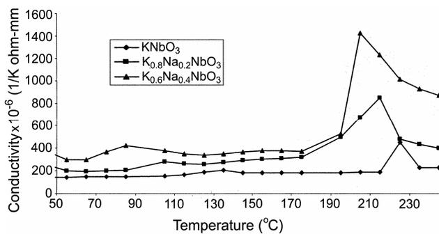
Fig. 6 — Variation of electrical conductivity with temperature for  $K_{1-x}Na_xNbO_3$  system at 1 MHz
