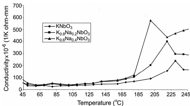
Fig. 7 — Variation of conductivity with temperature for  $K_{1-x}Na_xNbO_3$  system at 100 kHz
