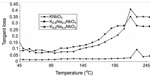
Fig. 5 — Variation of tangent loss with temperature for  $K_{1-x}Na_xNbO_3$  at 100 kHz
