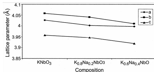
Fig. 1 — Composition dependence of lattice parameters
