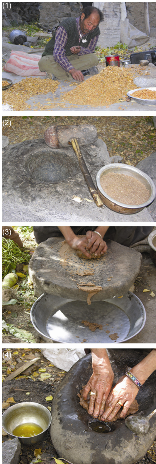
Fig. 1–Separation of kernel from broken shell; Fig. 2–Crushing of kernel in the mortar with hammer; Fig. 3–Grinding of kernel; Fig. 4–Extraction of oil.
