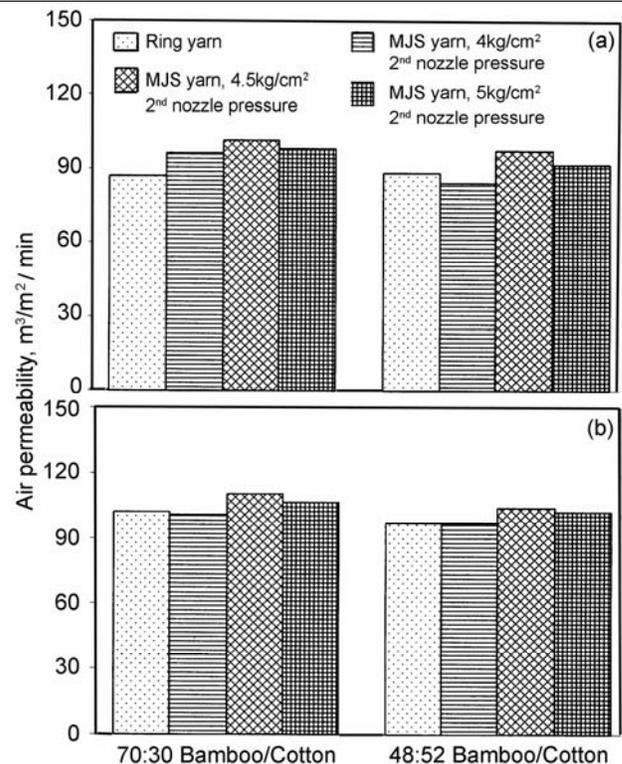
Fig. 1—Influence of process parameters on air permeability [(a) 19.6 tex; and (b) 14.7 tex]
