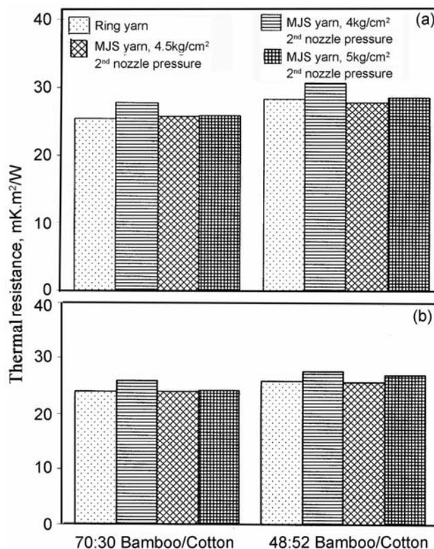
Fig. 2—Influence of process parameters on thermal resistance [(a) 19.6 tex; and (b) 14.7 tex]
