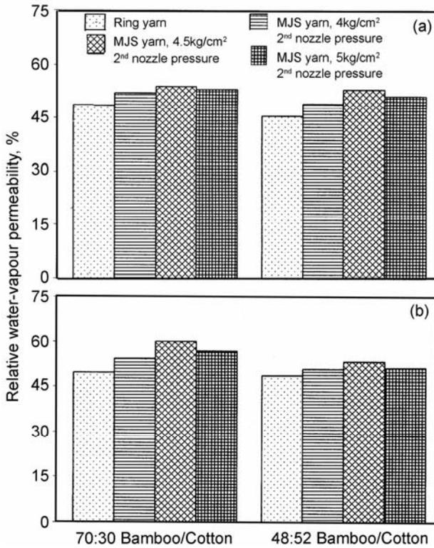
Fig. 3—Influence of process parameters on relative water-vapour permeability [(a) 19.6 tex; and (b) 14.7 tex]
