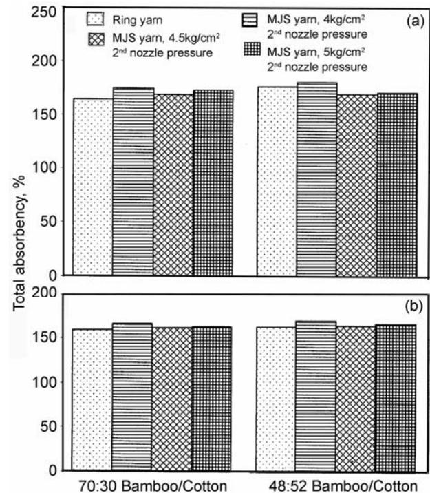
Fig. 5—Influence of process parameters on total absorbency [(a) 19.6 tex; and (b) 14.7 tex]
