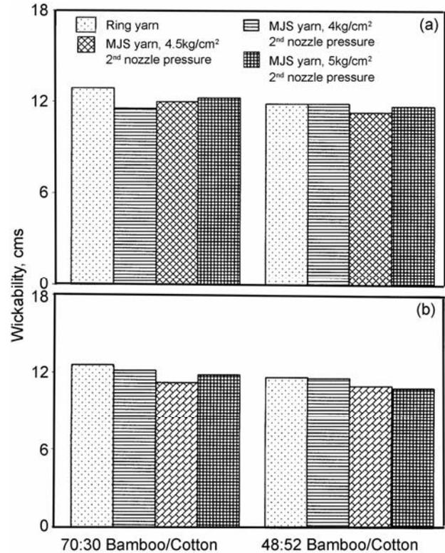
Fig. 4—Influence of process parameters on wickability [(a) 19.6 tex; and (b) 14.7 tex]
