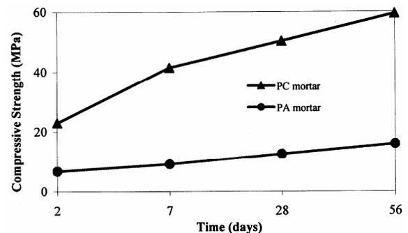
Fig. 1—Compressive strength of mortars versus time
