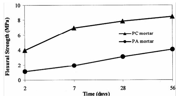
Fig. 2—Flexural strength of mortars versus time
