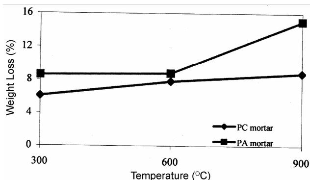
Fig. 5–Weight loss of mortars exposed to high temperatures
