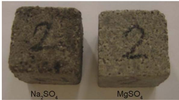
Fig. 6–Mortar specimens after 4-week immersion sulfate solutions
