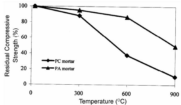
Fig. 3–Residual compressive strength after exposed to high temperatures
