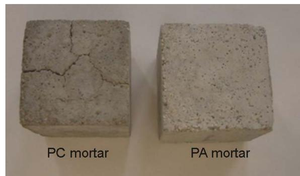
Fig. 4–Mortar specimens after exposure high temperatures (900°C)
