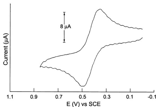
Fig. 3 — Cyclic voltammogram of (1) in  $\text{CH}_2\text{Cl}_2$ . [Cond.: dry  $\text{N}_2$  atmosphere; (1): 1.06 mmol dm<sup>-3</sup>;  $\text{Bu}_4\text{NClO}_4$ : 0.1 mol dm<sup>-3</sup>; glassy carbon working electrode; scan rate: 50 mV s<sup>-1</sup>].
