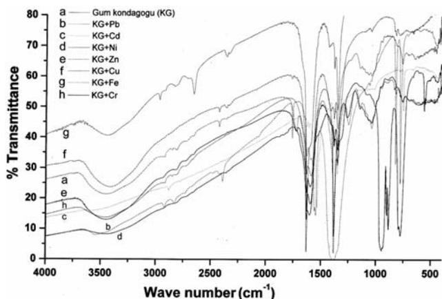
Fig. 4—FT-IR spectra of gum kondagogu before metal biosorption (a),  $Pb^{2+}$  loaded (b),  $Cd^{2+}$  loaded (c),  $Ni^{2+}$  loaded (d),  $Zn^{2+}$  loaded (e),  $Cu^{2+}$  loaded (f),  $Fe^{2+}$  loaded (g) and Cr loaded (h).
