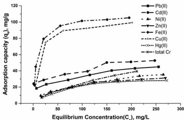
Fig. 1—Equilibrium isotherms of metal ions ( $Cd^{2+}$ ,  $Cu^{2+}$ ,  $Fe^{2+}$ ,  $Pb^{2+}$ ,  $Ni^{2+}$ ,  $Zn^{2+}$ ,  $Hg^{2+}$  and total Cr) and gum kondagogu interaction. Conditions: Initial metal ions concentrations, 25-300  $mg L^{-1}$ ; gum kondagogu dose, 1  $mg mL^{-1}$ ;  $pH$  5; temperature, 25°C; time of contact, 2 h.
