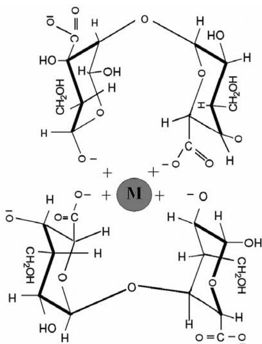
Fig. 5—Schematic diagram showing the cross-linking of a metal cation within gum kondagogu matrix ( $M^+ = Cd^{2+}, Cu^{2+}, Fe^{2+}, Pb^{2+}, Ni^{2+}, Zn^{2+}, Hg^{2+}$  and total Cr).
