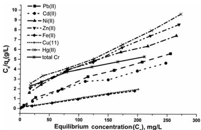
Fig. 2—Langmuir plots for metal ions ( $Cd^{2+}$ ,  $Cu^{2+}$ ,  $Fe^{2+}$ ,  $Pb^{2+}$ ,  $Ni^{2+}$ ,  $Zn^{2+}$ ,  $Hg^{2+}$  and total Cr) biosorption by gum kondagogu. Conditions: Initial metal ions concentrations, 25-300  $mg L^{-1}$ ; gum kondagogu dose, 1  $mg mL^{-1}$ ;  $pH$  5; temperature, 25°C; time of contact, 2 h.
