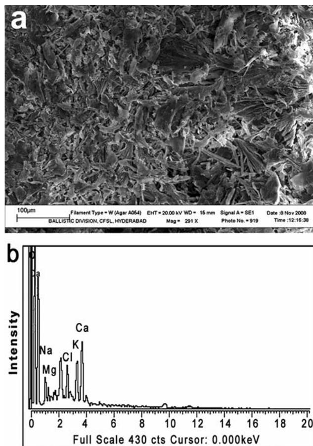
Fig. 3(a & b)—SEM micrograph of gum kondagogu before metal biosorption (a); EDXA spectrum of gum kondagogu before biosorption indicating various alkali and alkaline earth metals present (b).
