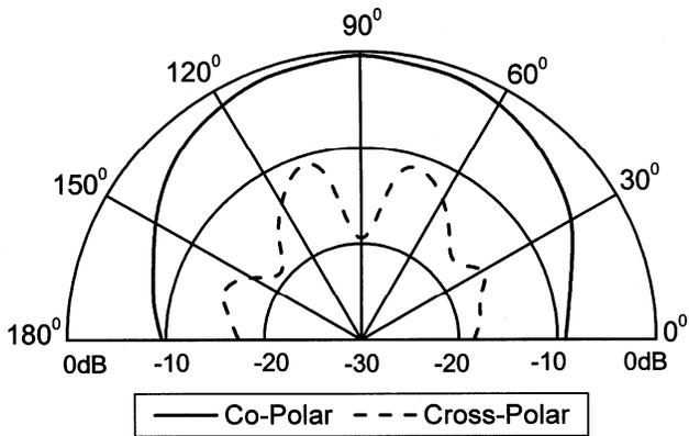
Fig. 3 — Radiation patterns of DRA<sub>1</sub> at 5.96 GHz
