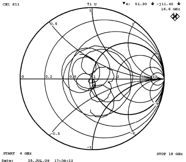
Fig. 7 — Input impedance profile of DRA<sub>4</sub>
