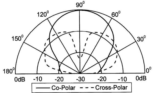
Fig. 5 — Radiation patterns of DRA<sub>3</sub> at 5.15 GHz
