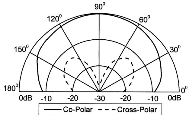
Fig. 6 — Radiation patterns of DRA<sub>4</sub> at 4.87 GHz
