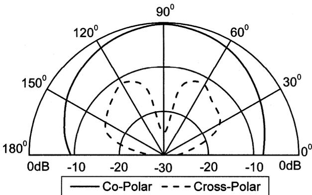
Fig. 4 — Radiation patterns of DRA<sub>2</sub> at 5.43 GHz
