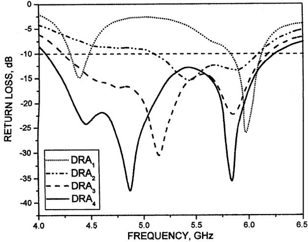
Fig. 2 — Return loss versus frequency of DRA<sub>1</sub>, DRA<sub>2</sub>, DRA<sub>3</sub> and DRA<sub>4</sub>
