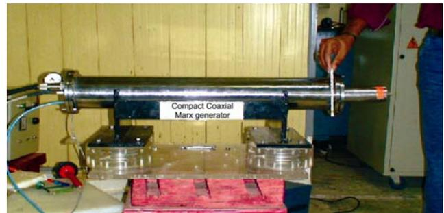
Fig. 13 — Assembled co-axial Marx generator
