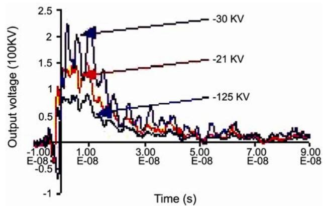
Fig. 19 — Output voltages at 100 Ω load
