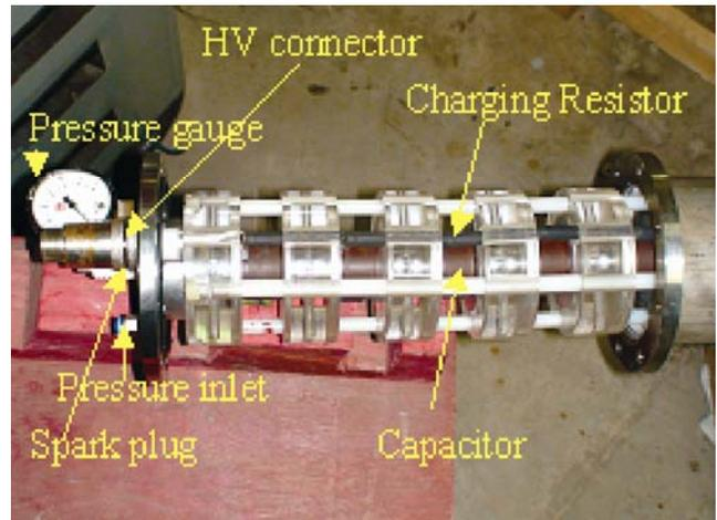
Fig. 11 — Internal view of co-axial Marx generator
