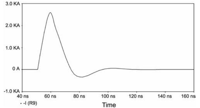
Fig. 8 — Simulated output current waveform at 71  $\Omega$
