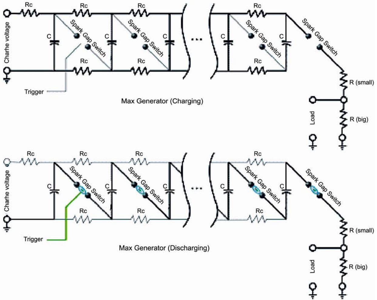
Fig. 1 — Good-let-Marx generator schematic
