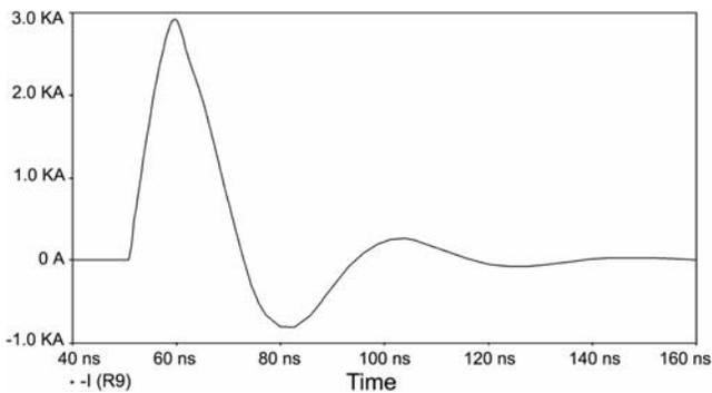
Fig. 6 — Simulated output current waveform at 50  $\Omega$
