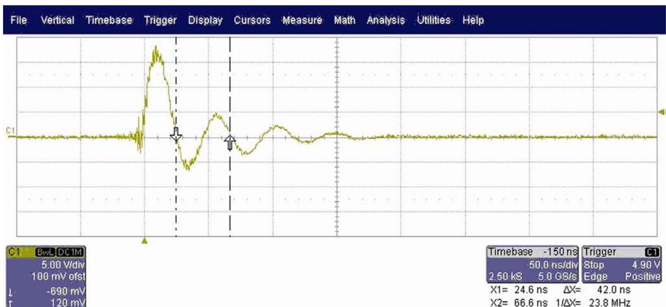
Fig. 15 — Short circuit test waveform
