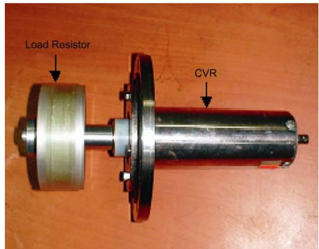
Fig. 12 — Pure ceramic resistive load 50Ω with CVR
