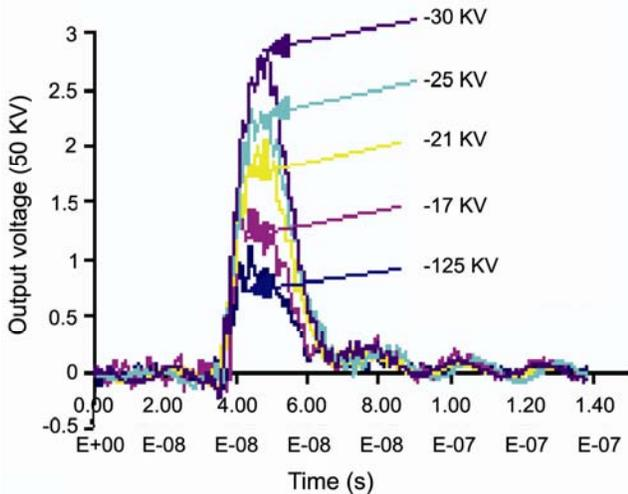
Fig. 18 — Output voltages at 50 Ω load
