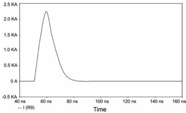
Fig. 10 — Simulated output current waveform at 100 Ω
