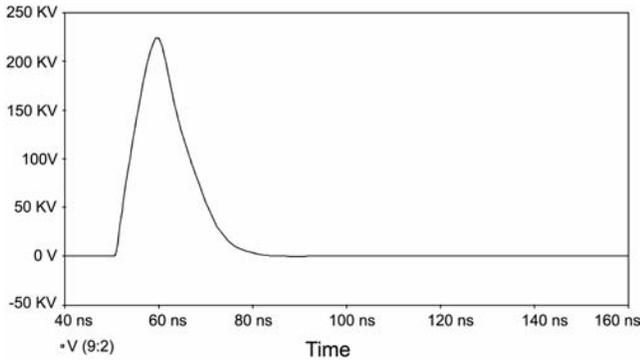
Fig. 9 — Simulated output voltage waveform at 100 Ω
