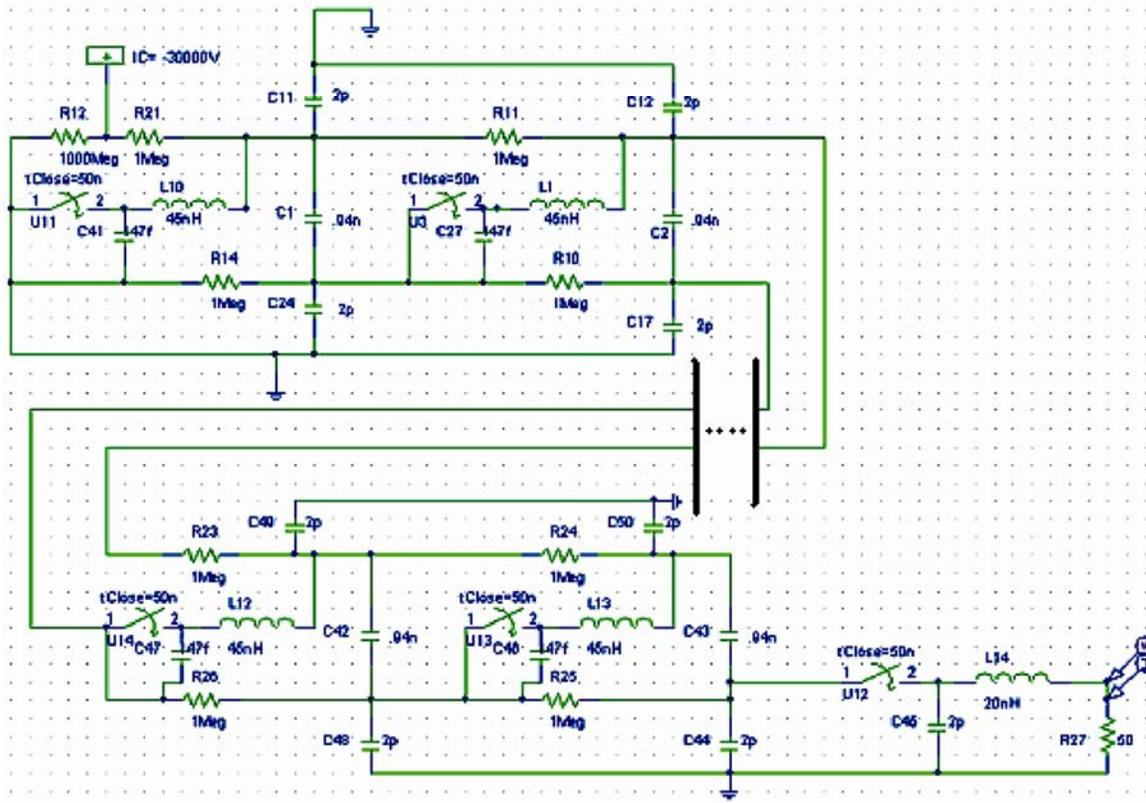
Fig. 4 — Marx generator simulation circuit
