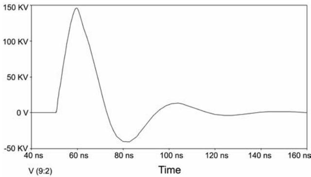
Fig. 5 — Simulated output voltage waveform at 50  $\Omega$
