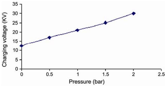
Fig. 17 — Charging voltage versus operating pressure
