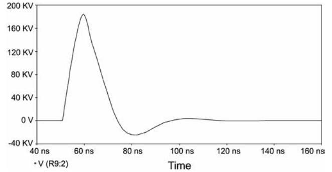
Fig. 7 — Simulated output voltage waveform at 71  $\Omega$
