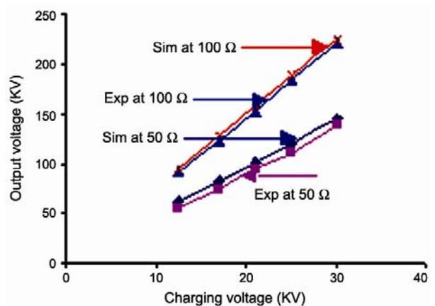
Fig. 20 — Experimental and simulated output voltages at 50 and 100 Ω
