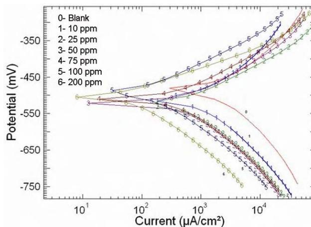
Fig. 2—Potentiodynamic polarization curve for MS in 1 M HCl in the absence and presence of different concentration of CBMTDT at 300 K
