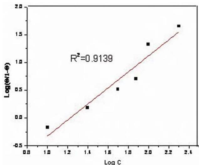
Fig. 6—Langmuir adsorption isotherm for MS in 1 M HCl at 300 K in the presence of CBMTDT
