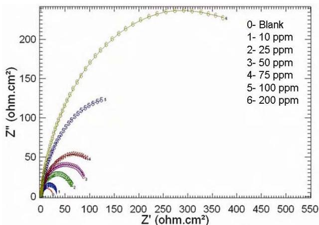
Fig. 4—Nyquist plots for MS in 1 M HCl in the absence and presence of different concentrations of CBMTDT at 300 K
