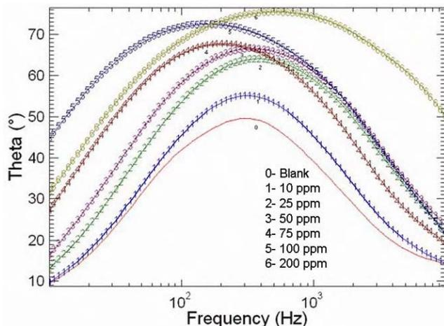
Fig. 5—Bode curves for MS in 1 M HCl in the presence of different concentrations of CBMTDT at 300 K
