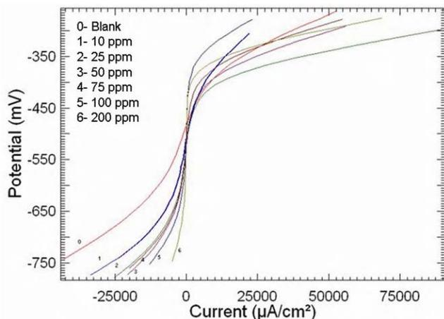
Fig. 3—Linear polarization curves for MS in 1 M HCl in the absence and presence of different concentrations of CBMTDT at 300 K
