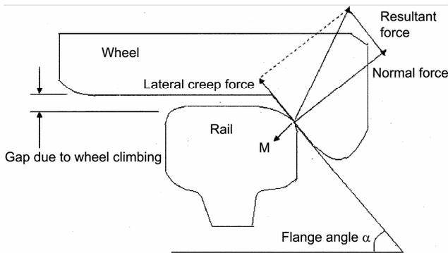
Fig. 6 — Inter-acting forces between rail gauge corner and wheel flange<sup>17</sup>
