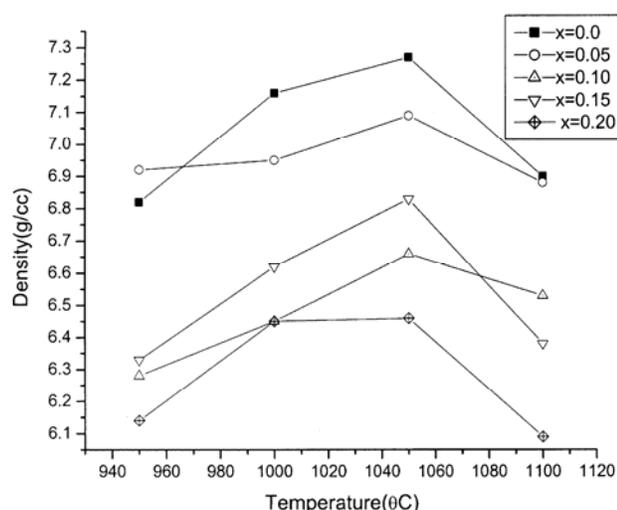
Fig. 3—Plot of density as a function of annealing temperature for Sr doped PbZrO<sub>3</sub> (Pb<sub>1-x</sub>Sr<sub>x</sub>ZrO<sub>3</sub>; x = 0, 0.05, 0.10, 0.15 and 0.20) ceramics
