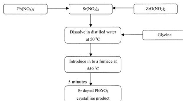
Fig. 1—Flow chart to prepare Sr doped with PbZrO<sub>3</sub> through glycine-nitrate combustion technique
