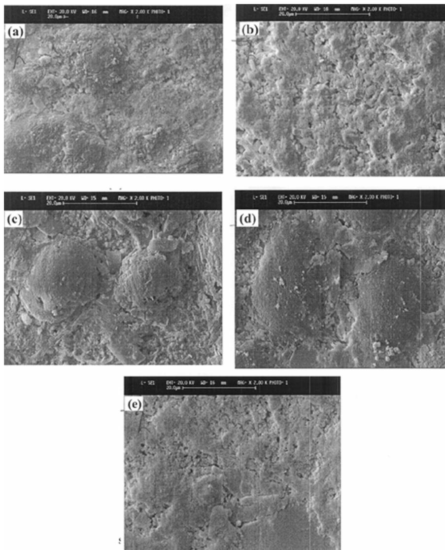
Fig. 5—SEM images of  $\text{Pb}_{1-x}\text{Sr}_x\text{ZrO}_3$  ceramics sintered at  $1050^\circ\text{C}$  for 2h : (a)  $x = 0$ , (b)  $x = 0.05$ , (c)  $x = 0.10$ , (d)  $x = 0.15$  & (e)  $x = 0.20$
