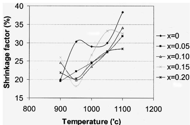
Fig. 4 (b)—The percentage shrinkage in volume of Sr doped  $\text{PbZrO}_3$  ( $\text{Pb}_{1-x}\text{Sr}_x\text{ZrO}_3$ ,  $x = 0, 0.05, 0.10, 0.15$  and  $0.20$ ) ceramics ( $\mu\text{m}$ ). From the above results, it is found that the
