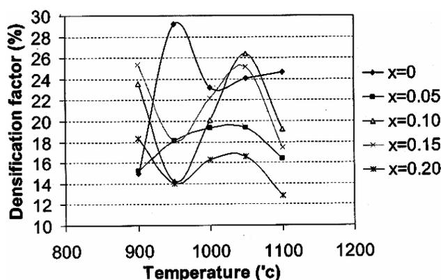
Fig. 4 (a)—The sintering behaviour pattern obtained on Sr doped PbZrO<sub>3</sub> (Pb<sub>1-x</sub>Sr<sub>x</sub>ZrO<sub>3</sub>; x = 0, 0.05, 0.10, 0.15 and 0.20) ceramics
