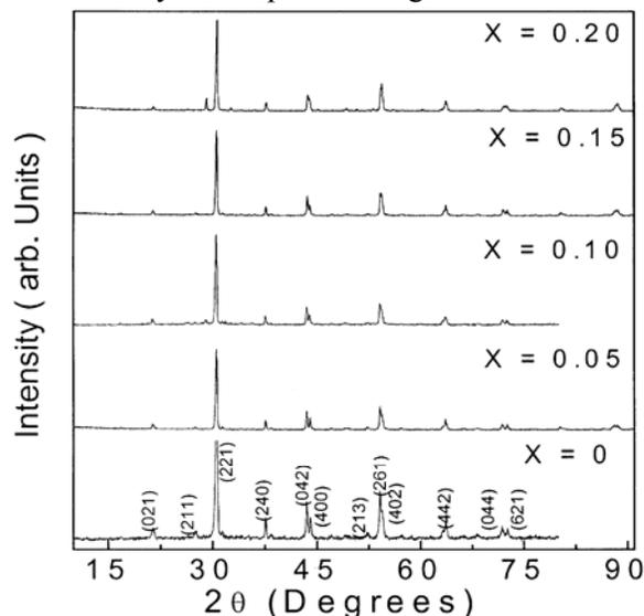
Fig. 2—XRD pattern obtained on Sr doped  $\text{PbZrO}_3$  ( $\text{Pb}_{1-x}\text{Sr}_x\text{ZrO}_3$ ;  $x = 0, 0.05, 0.10, 0.15$  and  $0.20$ ) ceramics
