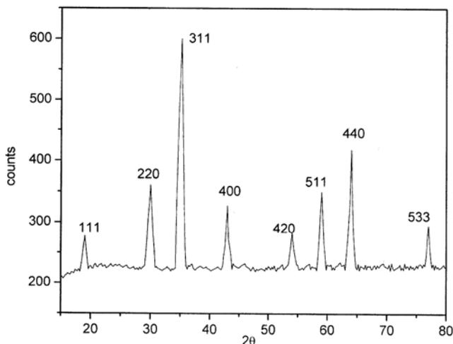
Fig. 2 — X-ray diffraction pattern of  $Mn_{0.4}Zn_{0.6}Al_{0.1}Fe_{1.9}O_4$  sintered at 500°C for 15 h
