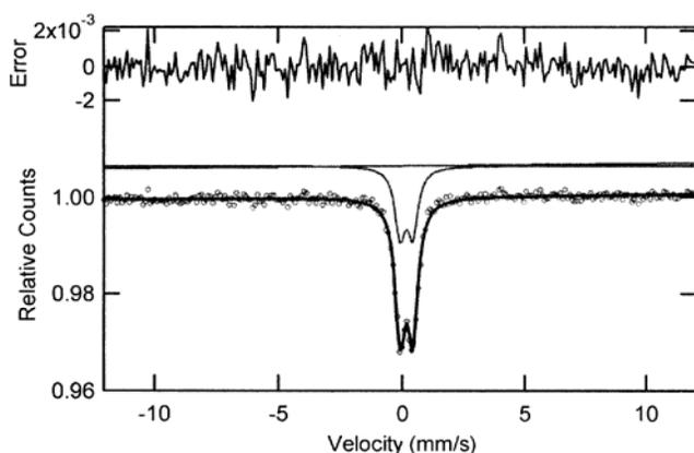
Fig. 10 — Room temperature Mössbauer spectrum for  $\text{Mn}_{0.4}\text{Zn}_{0.6}\text{Al}_{0.1}\text{Fe}_{1.9}\text{O}_4$  ferrite sample sintered at  $500^\circ\text{C}$
