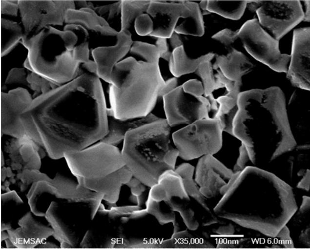
Fig. 4 — SEM of the fractured surface of Mn<sub>0.4</sub>Zn<sub>0.6</sub>Al<sub>0.1</sub>Fe<sub>1.9</sub>O<sub>4</sub> sintered at 500°C for 15 h
