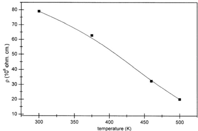
Fig. 9 — Variation of dc resistivity with temperature
