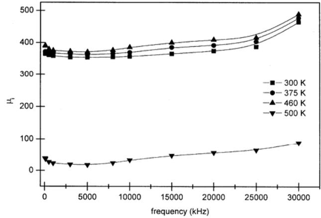
Fig. 5 — Variation of initial permeability,  $\mu_i$ , with frequency at different temperatures
