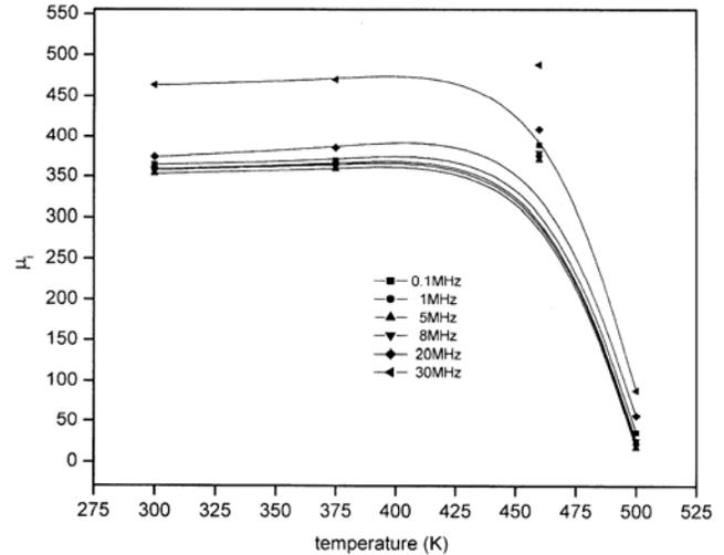
Fig. 6 — Variation of initial permeability,  $\mu_i$ , with temperature at different frequencies
