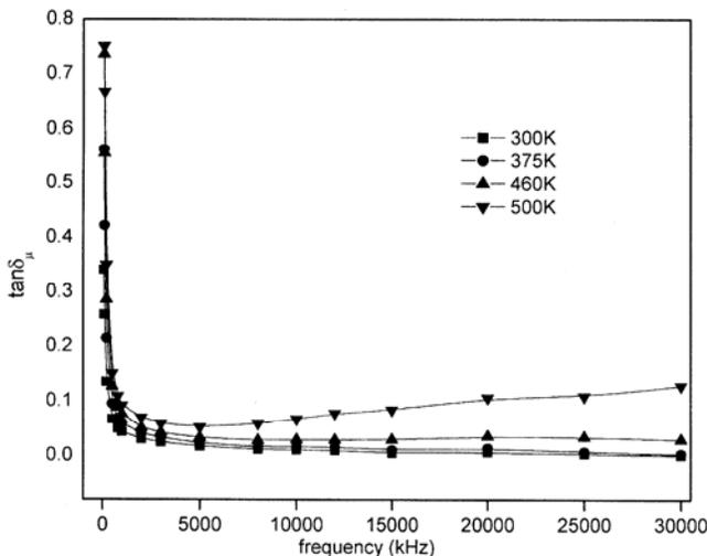
Fig. 7 — Variation of permeability loss factor,  $\tan\delta_\mu$ , with frequency at different temperatures
