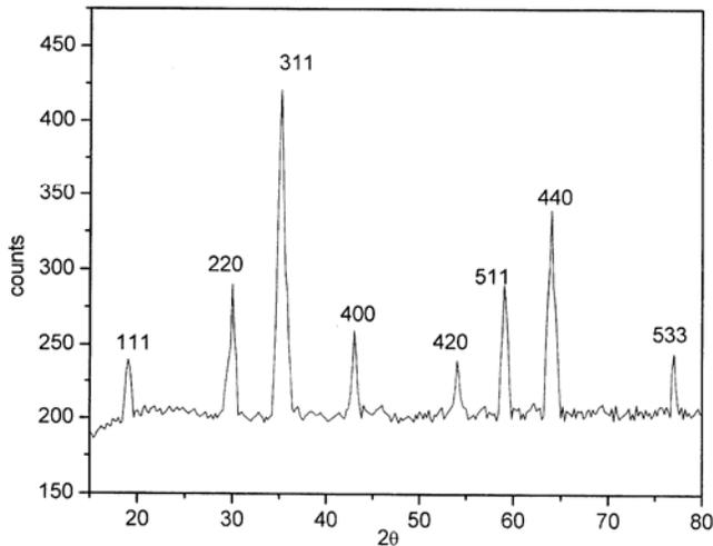
Fig. 1 — X-ray diffraction pattern of  $Mn_{0.4}Zn_{0.6}Al_{0.1}Fe_{1.9}O_4$  sintered at 200°C for 15 h
