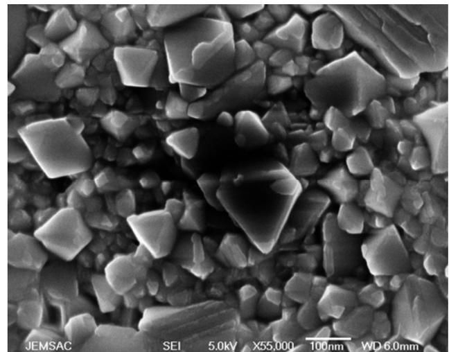
Fig. 3 — SEM of the fractured surface of  $Mn_{0.4}Zn_{0.6}Al_{0.1}Fe_{1.9}O_4$  sintered at 200°C for 15 h
