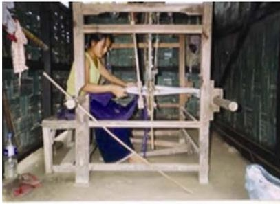
Fig.1 Throw shuttle loom
