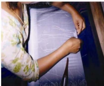
Fig.14 Way of inserting extra weft design
