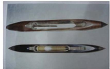
Fig.9 Spools used for fly shuttle loom
