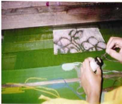
Fig.13 Designs transferred to warp yarn
