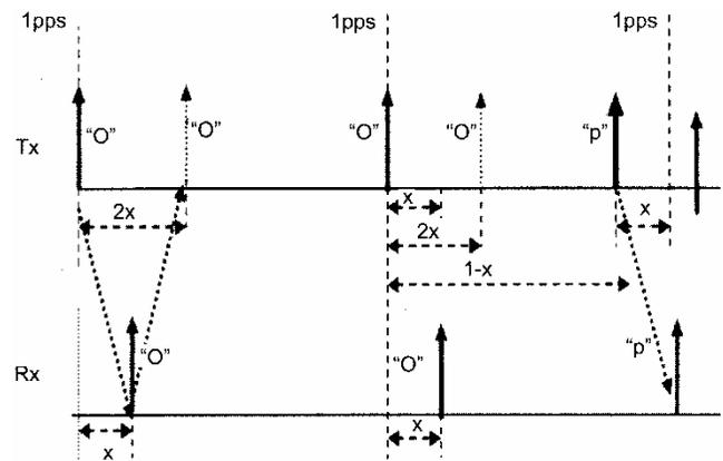
Fig. 7 — Plan of delay compensation
