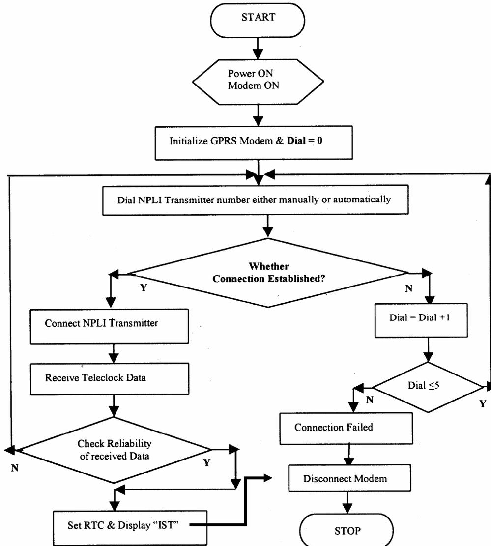
Fig. 4 — Algorithm to decipher correct data
