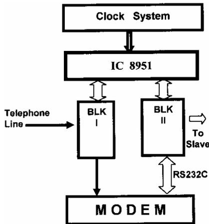
Fig. 3 — Functional diagram of Teleclock receiver. BLK I and BLK II are interfaces
