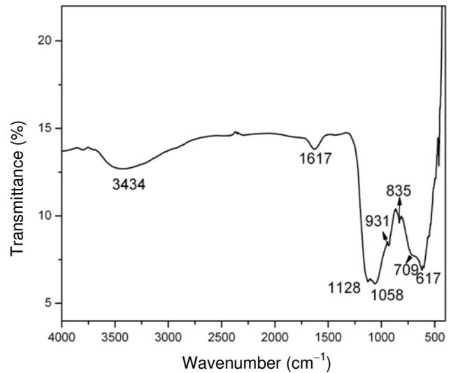
Fig. 3 — FTIR spectra of Kakching slag sample
