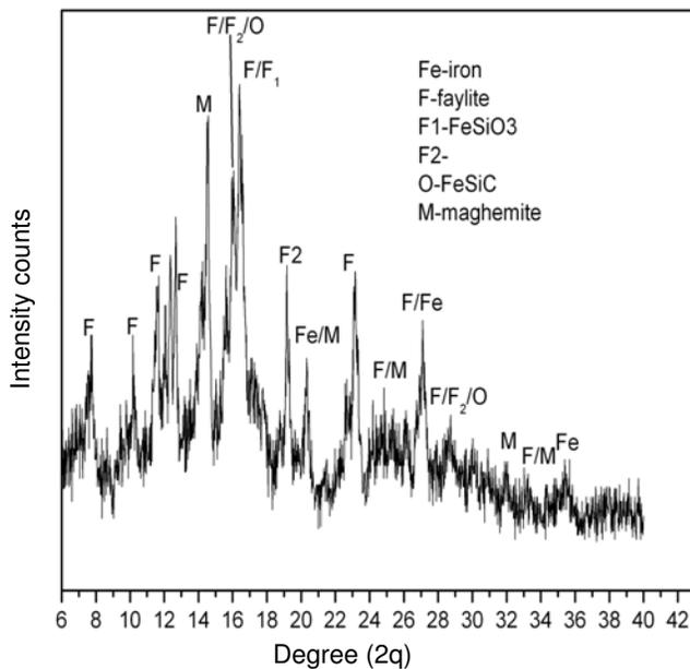
Fig. 2 — X ray diffraction pattern of Kakching slag sample: Fe-Iron card no – 6-696; F-Fayalite card no – 34-178; F1-FeSiO<sub>3</sub> card no – 12-284; F2- FeSiO<sub>4</sub> card no – 22-118; O-FeSi<sup>C</sup> card no – 26-798; M-Maghemite card no – 39-1346
